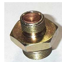
Copper restrictor fitted loose in the hose adapter. Hose end require more torque to prevent oil leak when securing hose.
