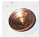
Copper restrictor fitted loose in the hose adapter. Hose end require more torque to prevent oil leak when securing hose.
